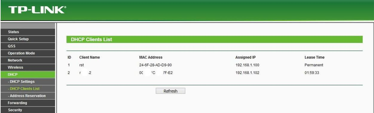
The screenshot shows the TP-LINK router web interface. The left sidebar contains a navigation menu with the following items: Status, Quick Setup, QSS, Operation Mode, Network, Wireless, DHCP (highlighted), - DHCP Settings, - DHCP Clients List (highlighted), - Address Reservation, Forwarding, Security, and Parental Control. The main content area is titled "DHCP Clients List" and contains a table with the following data:
