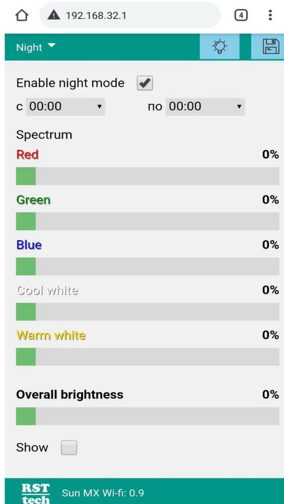
On this tab, you can configure the operating time of the backlight from ... to, as well as the spectrum by ticking the "Allow night mode"
